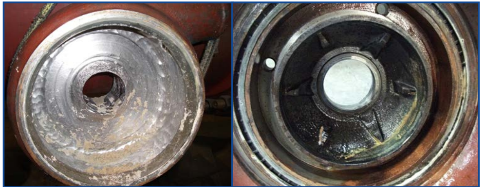
ON LEFT: Volute shows signs of severe wear. ON RIGHT: Cycloseal® backplate still has primer on it.
