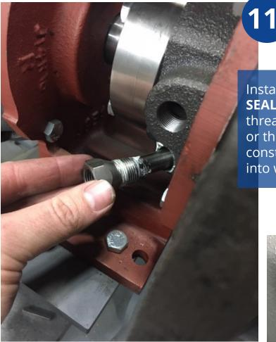
Install heater well using **PIPE THREAD SEALANT AND TEFLON TAPE** on threads. Do not over tighten heater well or the tapered thread will cause bore to constrict and heater probe will not insert into well.
