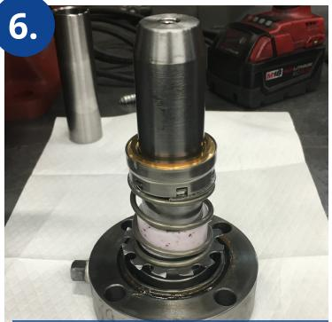
Place second seal with face up onto assembly spud. Be sure face is clean and dry, no oil residue.
