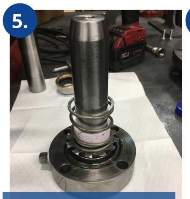
Place spring and seal spacer on spud.
