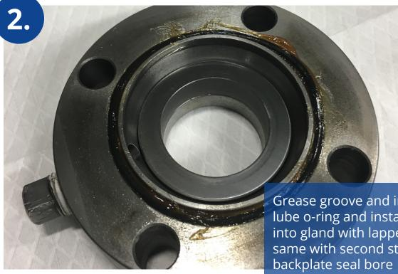
Grease groove and install o-ring in gland. lube o-ring and install stationary seal into gland with lapped **FACE UP**. Do the same with second stationary seal in the backplate seal bore
