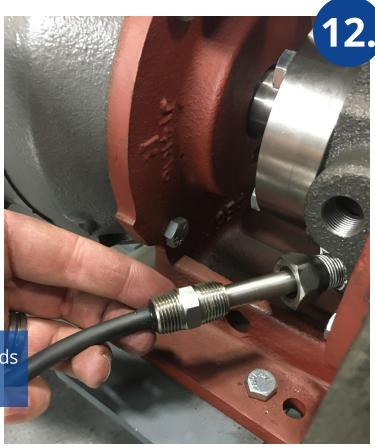
Install heater, apply ANTI-SEIZE to threads and probe as well to prevent sticking.
